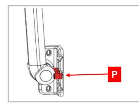
The lower ends of the arms can be attached from either the front or the side, depending on where the awning is being installed.
