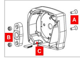
Attach the black piece that supports the end bearing to the side cover of the MICROBOX-300, on the opposite side to the one where the raising mechanism will be inserted. Use the DIN 7991 bolts (A) inserted from the outside of the cover, with the self-locking nuts (B) on the inside.
