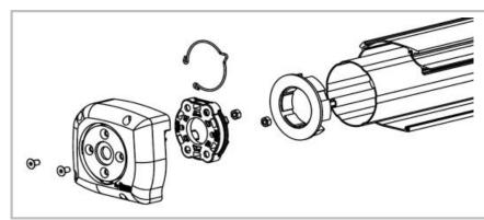
When inserting the motor into the HiPro bracket and attaching it with the attachment clip, first install the motor with the adapter crown and drive wheel as required for the chosen rolling tube, and place the whole assembly into the side cover. This allows some mobility that will make attachment easier.
