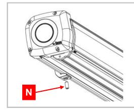
Now anchor the cassette to the various brackets by inserting and firmly tightening the stud (N).
