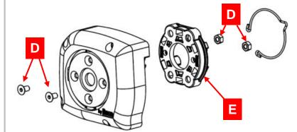
Prepare the side cover where the raising system will be located. If a motor is being used, attach the HiPro bracket (E) to this cover using the bolt kit (D) with reference number 11002035050. In this case, the bolts are inserted from the outside towards the inside, with the nuts being on the HiPro bracket side.
