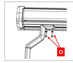
Attach the awning's arms to the attachment plates inserted in the front profile of the cassette, using the proper DIN 912 bolts (O). Do not tighten these all the way, so that the verticality can be adjusted once the lower ends of the arms are attached.
