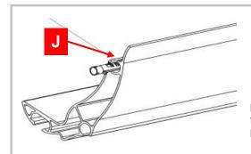
Insert the fabric hem rod into the cassette's front profile, or drop bar profile, and insert the plug (J) at both ends. These plugs hold the fabric in place and prevent horizontal movement when the fabric is being rolled up or extended.
