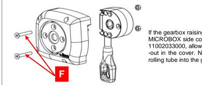
If the gearbox raising option has been chosen, attach this to the MICROBOX side cover using the bolt kit with reference number 11002033000, allowing the gearbox shaft to exit through the cut -out in the cover. Next, insert the bearing from the end of the rolling tube into the gearbox, with the fabric rolled up.
