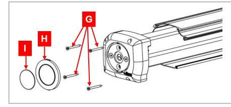
Next, attach the assembly to the profile using the bolts supplied (G), then attach the cover (H) and the Llaza sticker (I).
