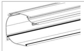
Once the profiles have been cut according to the measurements in the corresponding table, make sure that the cut is completely perpendicular in relation to the profile's length. Clean the ends of the profiles when they are received and remove any burrs produced during cutting, since these could affect proper assembly of the cassette.
